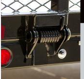
The Optional 4' Tall Rear Rampgate is equipped with Spring Assist- making lifting and using the gate easy and safe.
