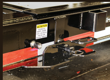
Tilt Latch & Cylinder Shut Off Valve
