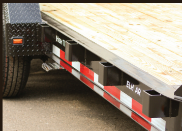
Heavy Duty 4" x 1/4" Bar Stake Pockets
