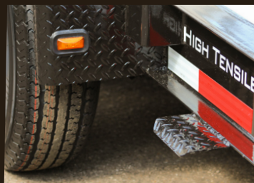
Step To Access Deck
