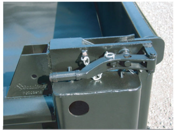
Pictured is a close view of the upper quick release hardware. This hardware makes it easy to quickly remove and reinstall the tailgate.
