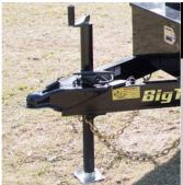
This 2,000# top wind jack is easy to use and works well on any surface. It is also bolted on for easy removal and replacement.
