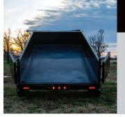
A sturdy 2" square tubing top rail, 24" tall 10-gauge sides and a single-piece, 10-gauge steel floor create a durable dump box.
