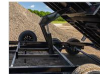
The Scissor-Lift Hydraulic System provides efficient lifting capabilities, a stable lifting platform and power-up, power-down, and gravity down functionality for quick dump cycles.
