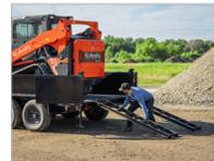
Standard Slide-In Ramps, Stabilizer Jacks, and D-Rings make it easy to load and secure the equipment you need for your job.
