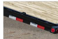
Benefit from enhanced cargo securement with our standard Rubrail, stake pockets and pipe spools. In addition to the built-in stake pockets, the Rubrail provides extra attachment points for securing your load. Customize your trailer further by adding optional D-rings.
