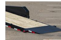
Our 30° Diamond plate knife edge tail makes it super-easy to load low clearance equipment like scissor lifts and fork lifts.
