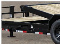
Our Gravity Tilt uses a hydraulic cylinder and proportioning valve to control the rate of tilt bed movement for additional safety when loading and unloading.
