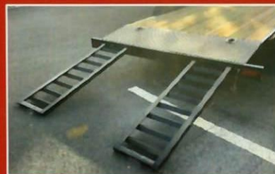
5' SLIDE OUT RAMPS PRESSURE TREATED WOOD DECK
