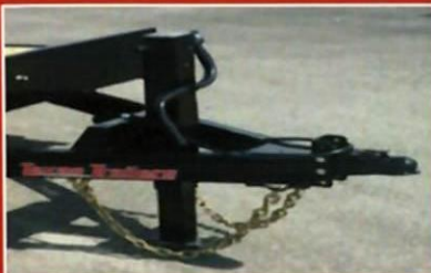
HD 12k DROP LEG SIDE WIND JACK ADJUSTABLE COUPLER
