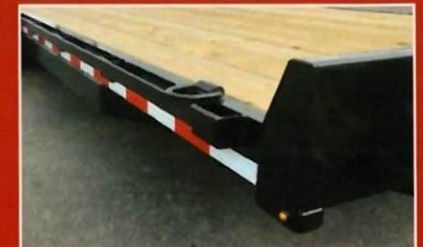
HD CHANNEL FULL WRAP A-FRAME STAKE POCKETS, RUBRAIL & D-RINGS
