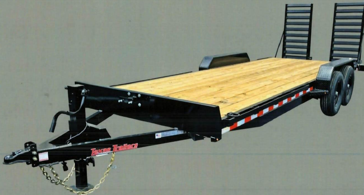
HD 12k DROP LEG SIDE WIND JACK ADJUSTABLE COUPLER
